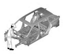
In order to perform anti-corrosion treatment, remove paint, grease and other substances from the new parts to be welded and the vehicle body, and then spray penetration weld primer.
