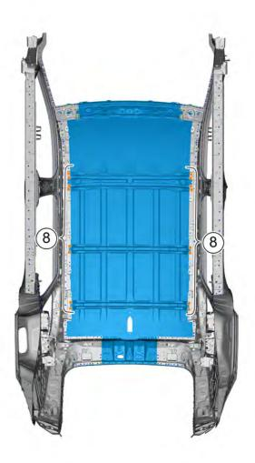
5. Mount the fixing points between the rear of panel roof assembly (without sunroof) and the left and right side wall assemblies.
