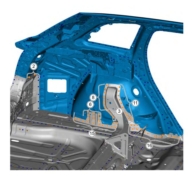
7. After drilling holes at the welding spots shown in the figure below, remove the fixing points between the left side wall assembly and the front cross beam assembly of roof and the rear crossmember assembly of roof.
