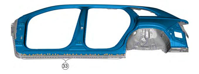
5. Mount the fixing points between the left side wall outer plate and the left A-pillar inner plate assembly and the left side wall rear drip rail assembly.
