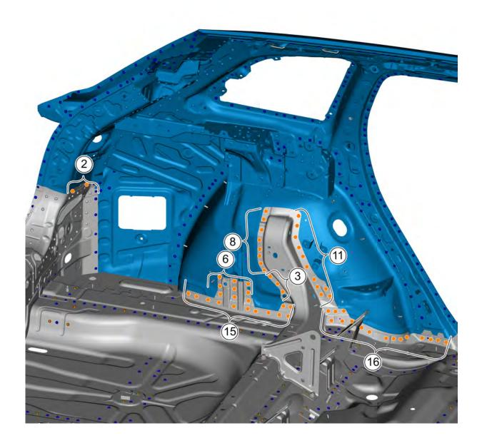
6. Mount the fixing points between the left side wall assembly and the rear wall panel assembly and the rear left side member assembly.
