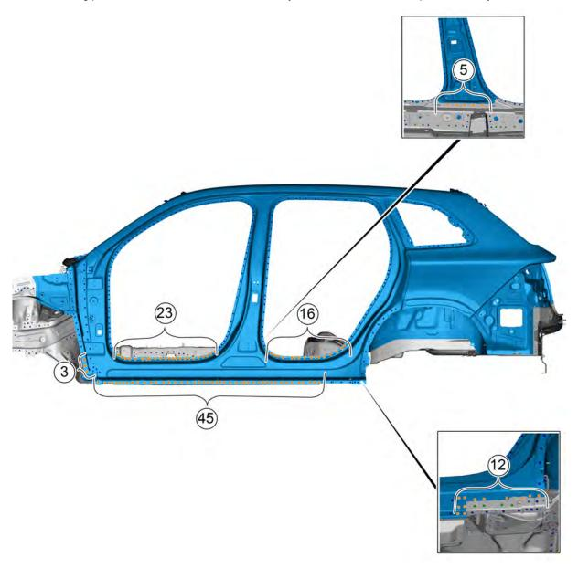
10. Mount the front connecting plate assembly of the left side wall.
