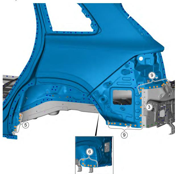
7. Mount the fixing points between the left side wall assembly and the left side member pulley cover assembly.
