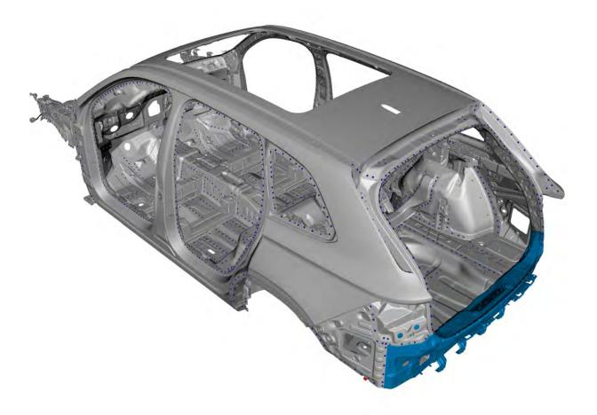
1. After drilling holes at the welding spots shown in the figure below, remove the fixing points between the rear wall panel assembly and the left side wall assembly & the rear floor assembly.
