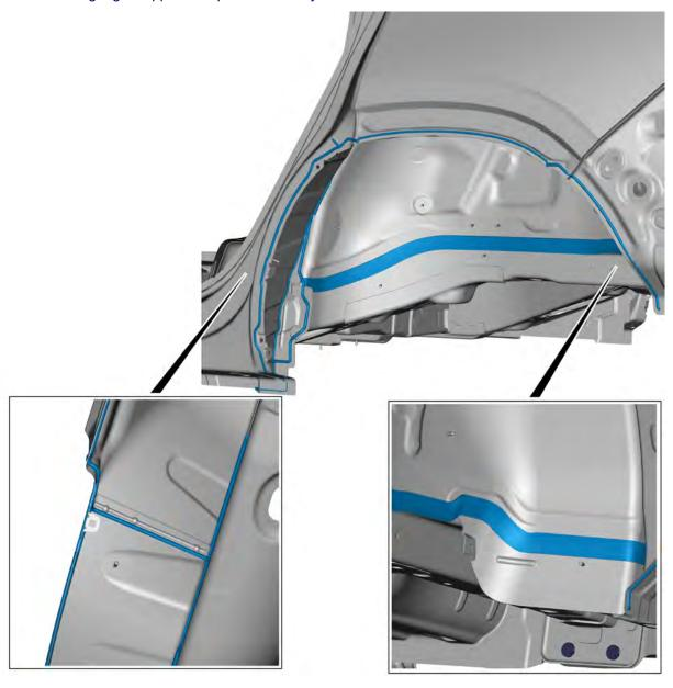
Sealant application positions on body floor
