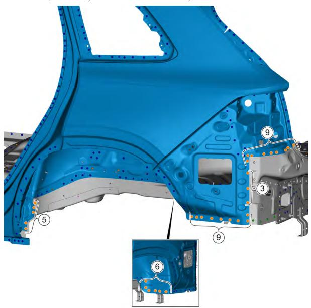
6. After drilling holes at the welding spots shown in the figure below, remove the fixing points between the left side wall assembly and the rear floor assembly.
