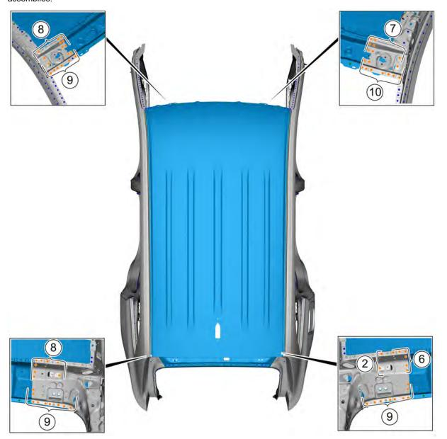
4. Mount the fixing points between the panel roof assembly (without sunroof) and the left and right side wall assemblies.
