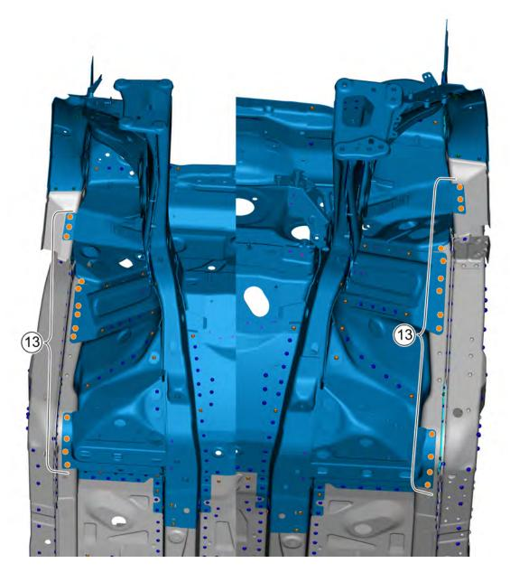
6. Mount the internal fixing points between the engine compartment assembly and the left and right A-pillar inner plate assemblies.
