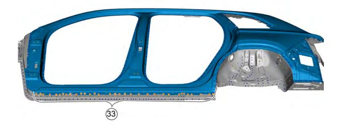
5. After drilling holes at the welding spots shown in the figure below, remove the fixing points between the left side wall outer panel assembly and the left side wall inner panel.
