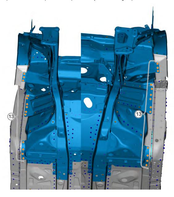
4. After drilling holes at the welding spots shown in the figure below, remove the external fixing points between the engine compartment and the left and right A-pillar inner panel assemblies.
