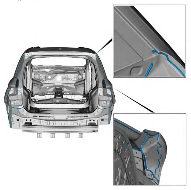
Sealant application positions on roof.
