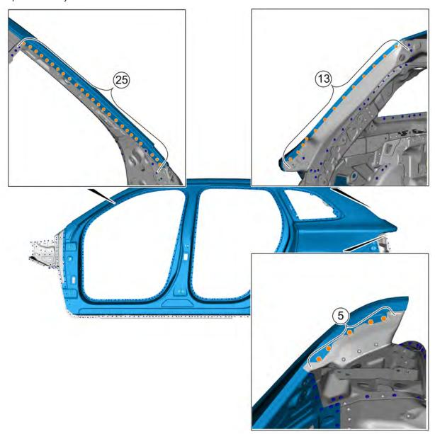
6. Mount the fixing points between the left side wall outer panel assembly and the left side wall inner panel.
