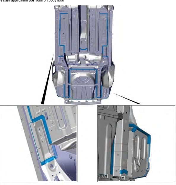
Sealant application positions on rear wall.
